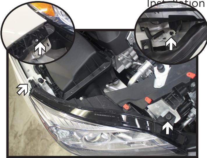
5. Using a 7MM socket, remove the four (4) screws from PS headlight. There are two (2) on the top side, one (1) along the side (left inset) and one (1) underneath (right inset). Disconnect the electrical line and set the headlight aside.
