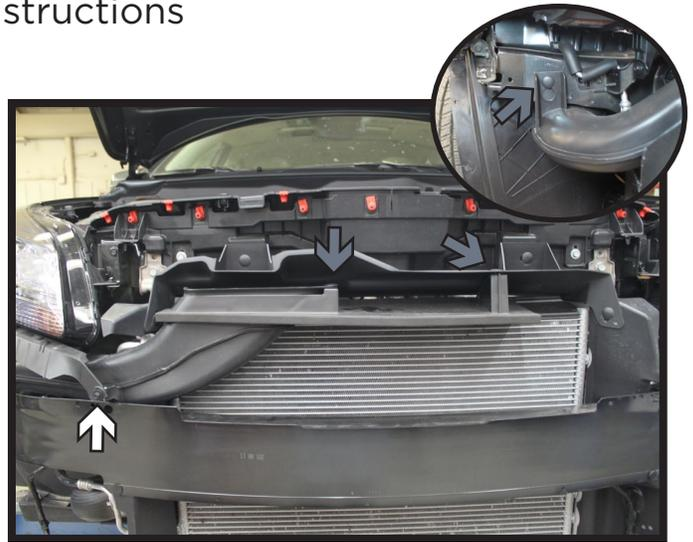
6. Using a 7MM socket, remove the screw from the front of the baffle (white). Then remove the rear push pin (inset) and the push pins on top towards the driver side (gray). Remove the baffle from the vehicle and set aside.
